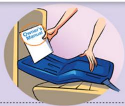
Conce installed, push and pull at belt path to ensure that the base (or car seat) doesn't move more than 1".
